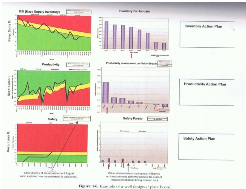
Figure 1-6. Example of a well-designed plant board.
